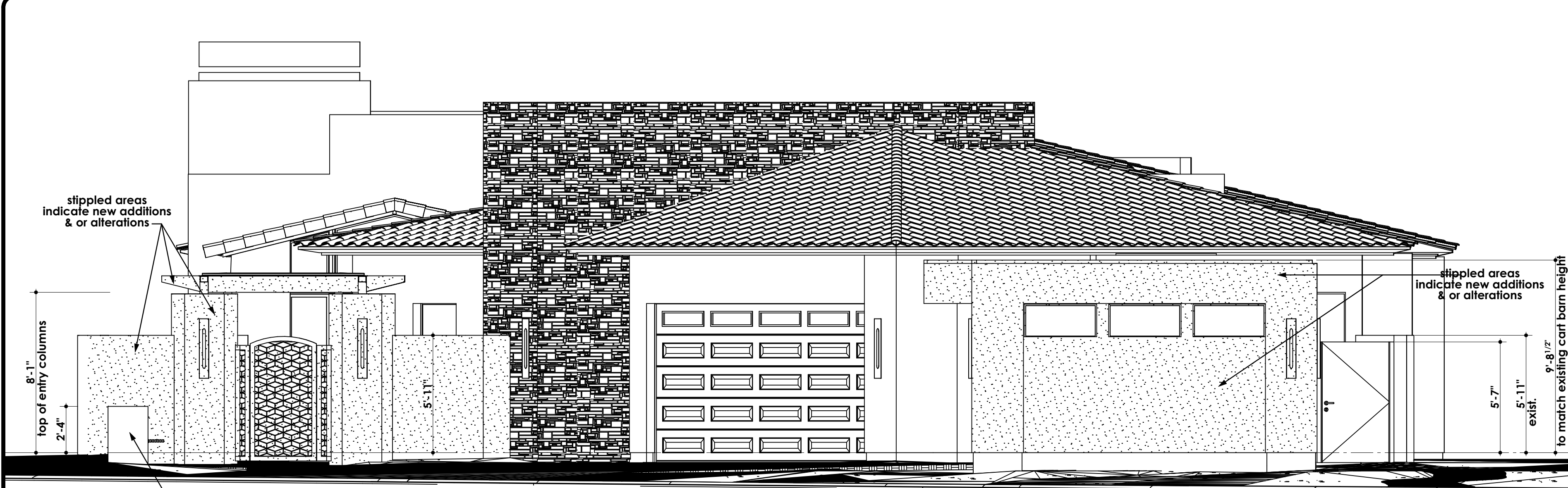
NEW CART BARN & ENTRY GATE (SOUTH PARTIAL EXTERIOR ELEVATION) DESERT TENAJA TRAIL
